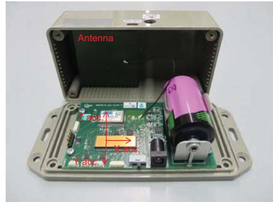
Fig. 3. Packaged accelerometer module with indication of axes.
